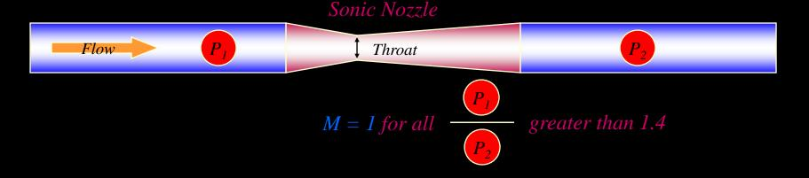
$\blacktriangleright M = 1$  represents choked condition, i.e. *condition of maximum mass flow rate*.
